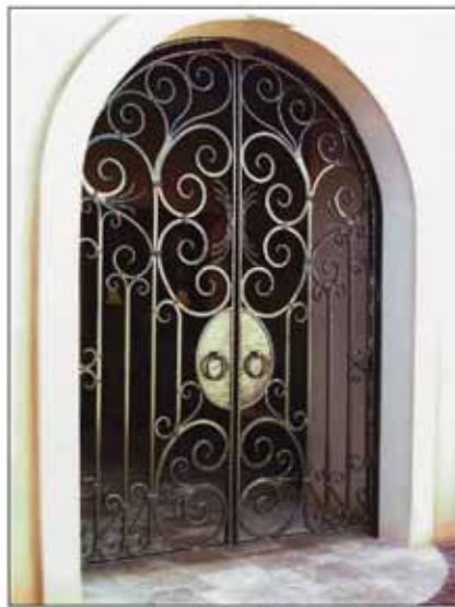
The company crafted this gate out of aluminum. The forged scrolls are made of 3/4" sq. forged stock. The frame is 1/2" x 1 1/2" heavy hammered stock, and the finish is bronze powder coat. Approx. labor time: 117 hrs.
